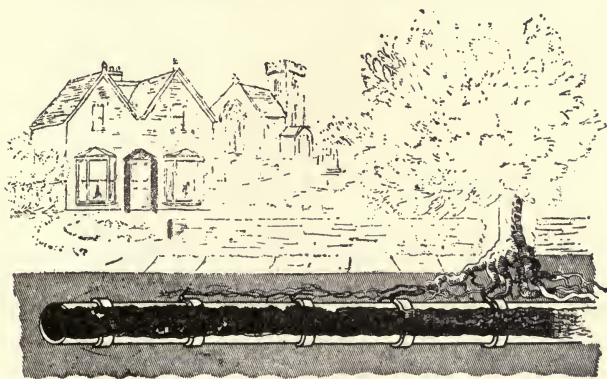
Fig. 625. Tree roots entering pipes laid with inferior mortar.
